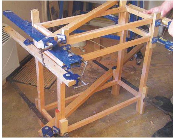
▲ Pic.9 Join the front and back rails together with end rails. Use a clamp across the diagonal to keep the frame square
